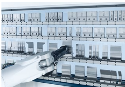
The ToolMaster Bend equips tools fully automatically.
