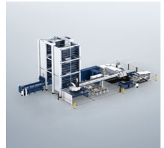
The TruMatic 7000 with a SheetMaster and double cart, indirectly connected to a TruStore 3030.
