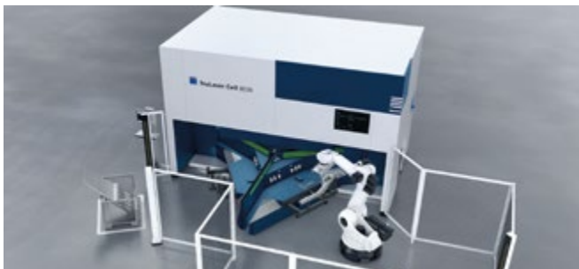
A rotary indexing table and robots keep cycle times to a minimum.
