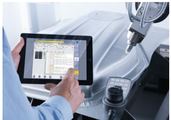
Quick program creation directly at the workpiece with the MobileControl App and teach panel.
