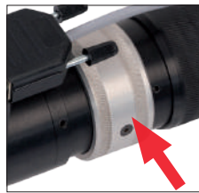
Instant switching between gap and contact welding
